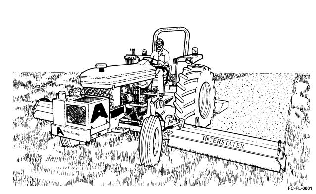
The Interstater is a revolutionary mowing system. Utilizing 2 side wings and 1 rear, you have ability to mow up to 20' across in on swath. Perfect for large areas of mowing including interstate highways and airport fields. A productive way to get a manicured cut in spaces there is high public visibility.
